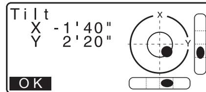
2. Check the position of the bubble of the circular level.
