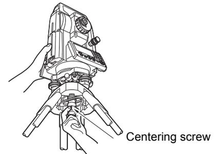
3. Looking through the optical plummet eyepiece, turn the optical plummet eyepiece to focus on the reticle.
