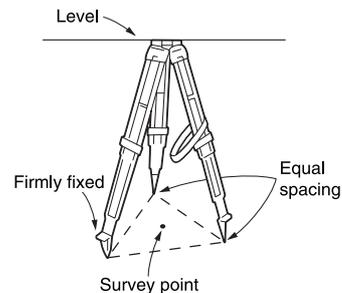
2. Place the instrument on the tripod head.
