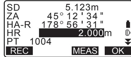
6. Confirm the measured result of the baseline defined from the line between the first target point and the second one.
