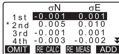
11. Press [RE\_CALC] to perform calculation again without the point designated in step 10. The result is displayed.
