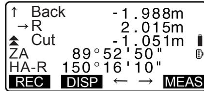
When the target is within measurement range, all four arrows are displayed.
