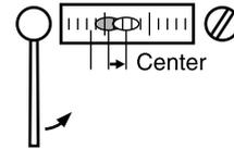
6. Rotate the top of the instrument and continue adjustments until the bubble remains centered for any position of the upper part.
