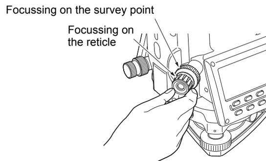
4. Adjust the levelling foot screws to center the survey point in the optical plummet reticle.
