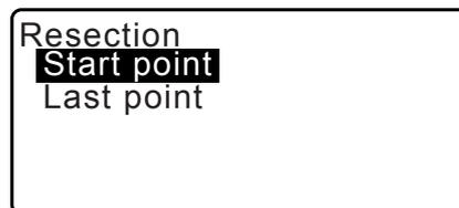
12. Press [OK] in the screen of step 9 to finish resection measurement. The instrument station coordinate is set.
