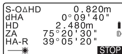
8. Move the prism forward and backward until the setting-out distance is 0 m. If S-O $\Delta$ HD is "+", move the prism toward yourself, if it is "-", move the prism away from yourself.
