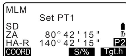
3. Input coordinates for the 1st target and press **[OK]**.
