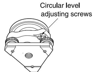
4. Adjust the adjusting screws until the tightening tension of the three screws is the same to align the bubble in the middle of the circle.
