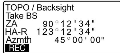
6. Sight the backsight and press **[REC]** in the screen of step 4, and set the following items.
