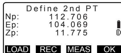
4. Enter azimuth angle (or horizontal distance) of the 1st point and 2nd point.
