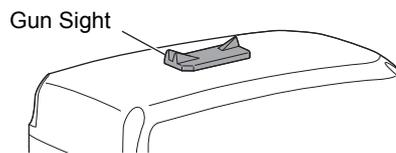
**Horizontal direction:** a position where you can see both the target and back sight at the center of the front sight's slit.
