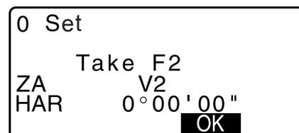
5. Turn the upper part through 180° and clamp it. Then set the telescope in the Face 2 position and accurately sight the same target.
