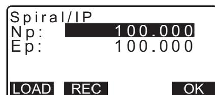
5. Enter the curve direction, parameter A, offset, and follow-up distance.
