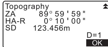
During the measurement for the second point and thereafter, if: (1) Number of distance sets (No. of SETs) is set to "1"; (2) Number of distance readings (No. of Obs) is set to "1"; and (3) RL observation (F1/F2 Obs) is set to "No"; **[OFFSET]** is displayed. Pressing **[OFFSET]** enables offset measurement of the target point.
