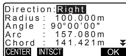
10. Press **[OK]** on the screen of step 9 to define the arc. <Set-out arc> is displayed. Move to setting-out arc measurement.
