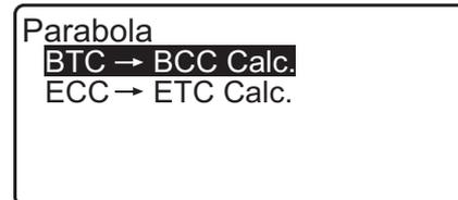
3. Input the coordinates of the BTC point (reference point). Press **[OK]** to set the input values.
