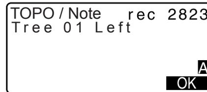
3. After inputting the note data, press **[OK]** to return to <TOPO>.
