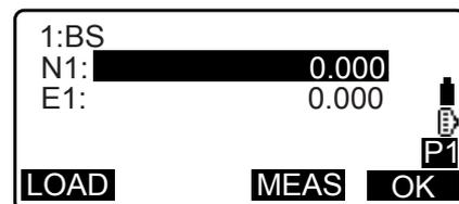
5. Input horizontal angle and distance from instrument station, then press **[OK]**. Coordinates for the target point are displayed.
