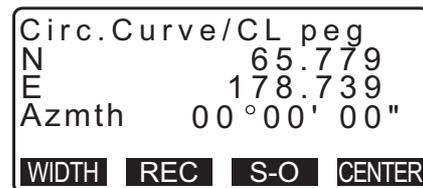
7. Press **{ESC}** twice to finish Circular Curve calculation and return to <Road>.
