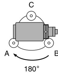
4. Correct half of the bubble displacement using levelling foot screw C.
