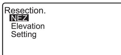
4. Measure the first known point in Face 1. "R" is displayed in the screen title. Press **[MEAS]** to start measuring. The measurement results are displayed on the screen.
