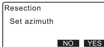
Pressing **[OK]** sets the direction angle and instrument station data, and then returns to <Coord.>.
