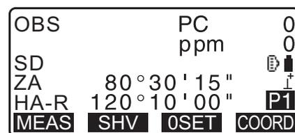
When measurement starts, EDM information (distance mode, prism constant correction value, atmospheric correction factor) is represented by a flashing light.
