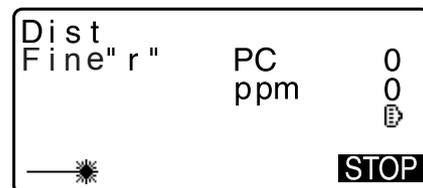
A short beep sounds, and the measured distance data (SD), vertical angle (ZA), and horizontal angle (HA-R) are displayed.
