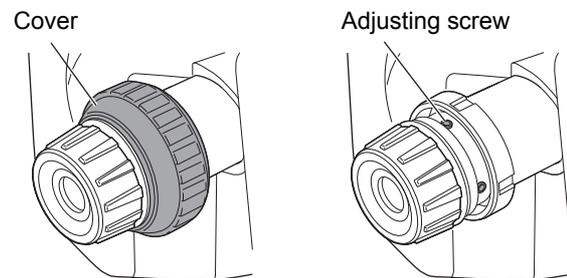
5. Turn the 4 adjusting screws of the optical plummet to adjust the remaining half of the deviation using hexagonal wrench (1.3 mm) as shown below.
