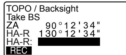
5. Sight the backsight and press **[REC]** in the screen of step 4, and set the following items.
