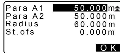
6. Press **[OK]** in the screen shown in step 5 to calculate the coordinates and follow-up distance of the KA1 point, KE1 point, KE2 point, and KA2 point. The results are then displayed on the screens shown here. Press **[RIGHT]**/**[LEFT]** to switch between <IA&Tangent/KA1>/<IA&Tangent/KE1>/<IA&Tangent/KE2>/<IA&Tangent/KA2>.
