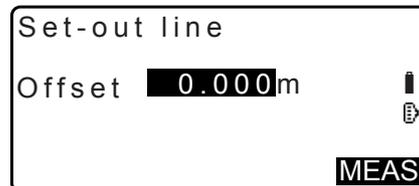
3. Sight the target and press **[MEAS]** on the screen of step 2. The measurement results are displayed on the screen. Press **[STOP]** to stop the measurement.
