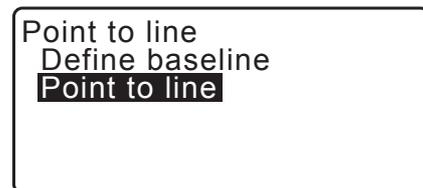
3. Collimate the target point and press **[MEAS]**. The measured result is displayed.
