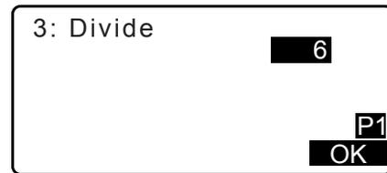
6. Coordinates for each dividing point are displayed on consecutive screens. To switch between result screens, press **[▶]/[◀]**. Press **[OK]** to return to the screen in step 3 and continue measurement as necessary.
