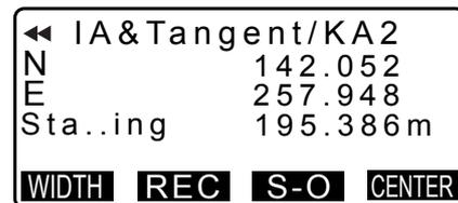
7. In the screens for the KA1 point, KE1 point, KE2 point, and KE2 point that have been found, press **[CENTER]** to move to centerline peg settings.
