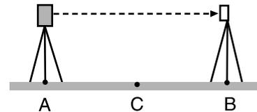
2. Precisely measure the horizontal distance between point A and point B 10 times and calculate the average value.
