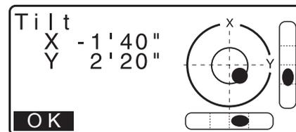
3. Carefully level the instrument and press **[OK]**.
