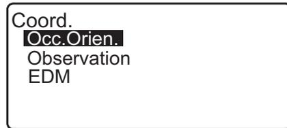
4. In <Coord>, select "Observation". Pressing **[MEAS]** will start measurement, and the coordinate value of the target will be displayed. Press **[STOP]** to quit measurement.
