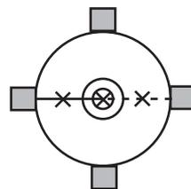
6. Check to make sure that the survey point remains centered on the reticle even if the upper part of the instrument is rotated.
