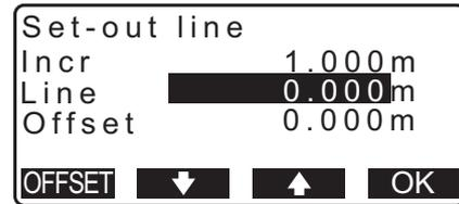
3. Press **[OK]** on the screen of step 2. The coordinate value of the required point is calculated and displayed.
