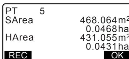
9. Press **[REC]** in the screen of step 8 to record results and return to <Menu>. Press **[OK]** to return to <Menu> without recording results.
