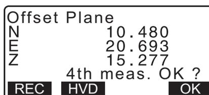
7. After finishing measurement, press **[OK]** in the screen of step 6 to return to <Offset>.
