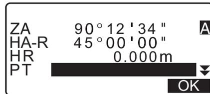
7. Press **[OK]** to record backsight station data. Known point data and angle measurement data are recorded at the same time. <TOPO> is restored.
