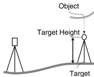
2. After inputting the target height, accurately sight the target.
