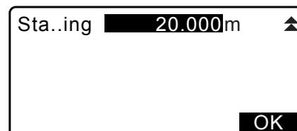
6. Press **[OK]** in the screen shown in step 5 to calculate the center peg coordinates. The coordinates are then displayed in this screen.
