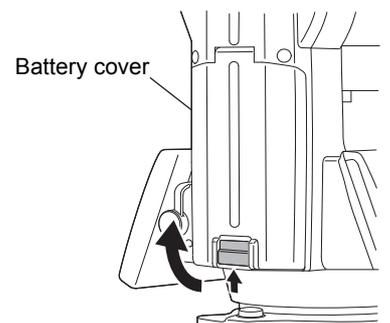
2. Checking the terminal side on the battery, insert the battery as shown.
