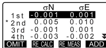
10. If there are problems with the results of a point, align the cursor with that point and press [OMIT]. "\*" is displayed on the left of the point. Repeat for all results that include problems.
