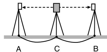
4. Precisely measure the horizontal distances CA and CB 10 times each and calculate the average value for each distance.
