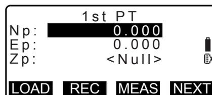
5. Press **[OK]**. The coordinate value of the intersection point is calculated and displayed.
