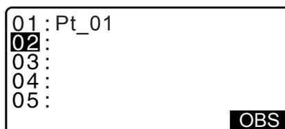
7. Repeat steps 4 to 6 until all points have been measured. Points on an enclosed area are observed in a clockwise or counterclockwise direction. For example, the area specified by entering point names 1, 2, 3, 4, 5 or 5, 4, 3, 2, 1 implies the same shape. After all known points necessary to calculate the surface area have been observed, **[CALC]** is displayed.
