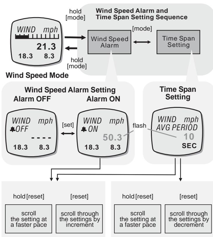
To Set the Wind Speed Alarm, and Time Span for Average Wind Speed Calculation
