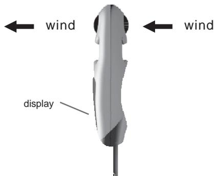
**Point the Propeller towards the wind direction**
